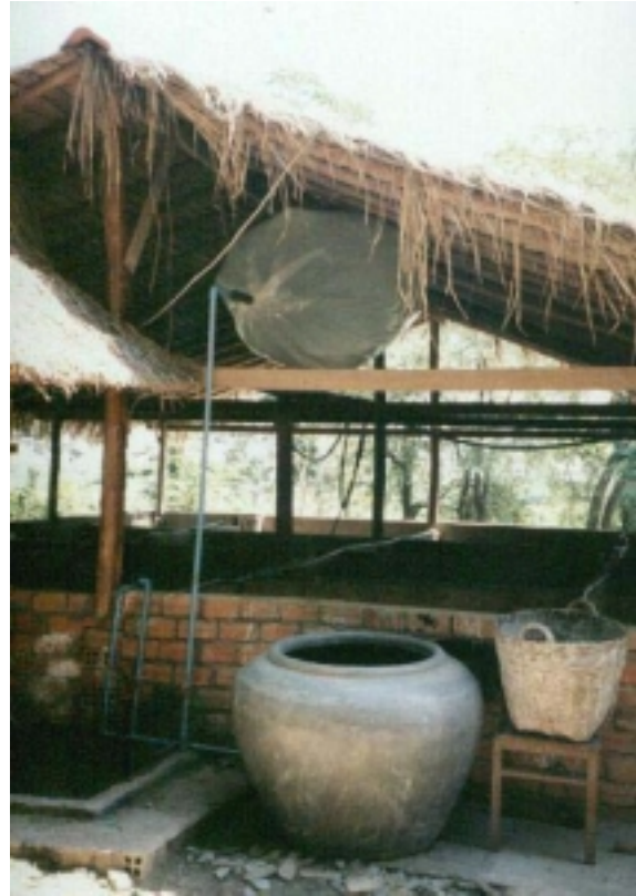
This hybrid biogigester in Cambodia, uses pig dung as an energy source.
