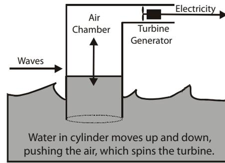
tower built into a cliff produces electricity for about four cents a kWh using this method. The wail of the fast-spinning turbines, however, can be heard for miles.
